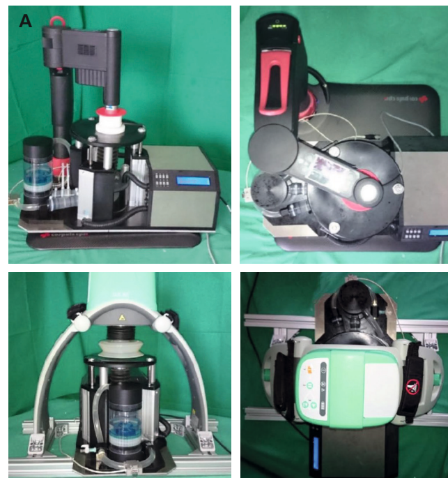
Fig. 1. a Two different chest compression devices interacting with a physical thorax model. Upper pictures corpuls cpr ; lower pictures LUCAS II (backboard replaced with metal frame for better contact with model). b Schematic of the physical patient model: 1 air-compression pump; 2 spring; 3 pneumatic piston; 4 variable gaiter; 5 single-chamber heart; 6 reservoir with bubble trap; 7 computer-controlled valve
